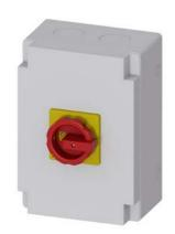
SENTRON, Switch disconnector 3LD, emergency switching-off switch, 3- pole, lu: 100 A, operating power / at AC-23 A 400 V: 37 kW, Molded plastic encapsulation for inch cable gland, rotary operating mechanism, red/yellow
