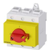
SENTRON, Switch disconnector 3LD, emergency switching-off switch, 3- pole, lu: 100 A, operating power / at AC-23 A 400 V: 37 kW, installation in distribution boards, knob-operated mechanism, Red / yellow, handle direct at the switch
