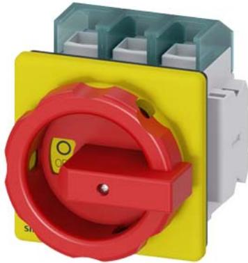
SENTRON, Switch disconnecter 3LD, emergency switching-off switch, 3- pole, Iu: 100 A, operating power / at AC-23 A 400 V: 37 kW, front-mounted, 1 NC, 1 NO, rotary operating mechanism, Red / yellow, 4-hole mounting of the handle
