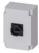
SENTRON, Switch disconnector 3LD, main switch, 6-pole, lu: 63 A, Operating power / at AC-23 A at 400 V: 22 kW, molded-plastic encapsulation for metric screw connection, 1 NC, 1 NO, rotary operating mechanism, black
