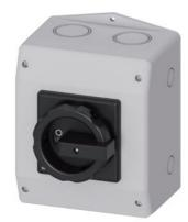
SENTRON, Switch disconnector 3LD, main switch, 3-pole, lu: 63 A, Operating power / at AC-23 A at 400 V: 22 kW, molded-plastic encapsulation for inch cable gland, rotary operating mechanism, black
