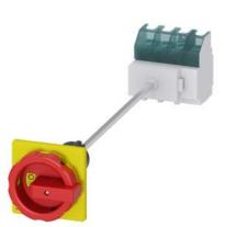
SENTRON, Switch disconnector 3LD, emergency switching-off switch, 4- pole, lu: 63 A, operating power / at AC-23 A 400 V: 22 kW, floor mounting with door coupling, rotary operating mechanism, Red / yellow, central mounting 22.5 mm of the handle
