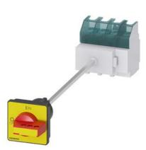
SENTRON, switch disconnector 3LD, EMERGENCY OFF switch, 4-pole, lu: 63 A, Operating power / at AC-23 A at 400 V: 22 kW, floor mounting with door coupling, defeatable knob-operated mechanism, red/yellow, 4-hole mounting of the handle
