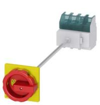
SENTRON, Switch disconnector 3LD, emergency switching-off switch, 4- pole, lu: 63 A, operating power / at AC-23 A 400 V: 22 kW, floor mounting with door coupling, rotary operating mechanism, Red / yellow, 4-hole mounting of the handle
