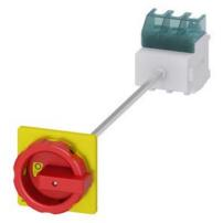
SENTRON, Switch disconnector 3LD, emergency switching-off switch, 3- pole, lu: 63 A, operating power / at AC-23 A 400 V: 22 kW, floor mounting with door coupling, rotary operating mechanism, Red / yellow, 4-hole mounting of the handle
