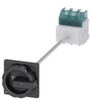
SENTRON, Switch disconnector 3LD, main switch, 3-pole, lu: 63 A, Operating power / at AC-23 A at 400 V: 22 kW, floor mounting with door coupling, rotary operating mechanism, black, 4-hole mounting of the handle
