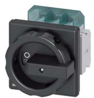
SENTRON, Switch disconnector 3LD, main switch, 3-pole, lu: 63 A, Operating power / at AC-23 A at 400 V: 22 kW, front-mounted, 1 NC, 1 NO, rotary operating mechanism, black, 4-hole mounting of the handle
