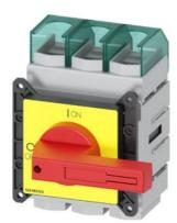
SENTRON, Switch disconnector 3LD, emergency switching-off switch, 3- pole, lu=250 A, operating power / at AC-23 A 400 V: 132 kW, front-mounted, knoboperated mechanism, red/yellow, 4-hole mounting of the handle
