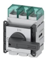
SENTRON, Switch disconnector 3LD, main switch, 3-pole, lu=250 A, Operating power / at AC-23 A at 400 V: 132 kW, front-mounted, knob-operated mechanism, black, 4-hole mounting of the handle
