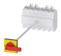
SENTRON, Switch disconnector 3LD, emergency switching-off switch, 6- pole, lu: 160 A, operating power / at AC-23 A 400 V: 75 kW, floor mounting with door coupling, knob-operated mechanism, red/yellow, 4-hole mounting of the handle
