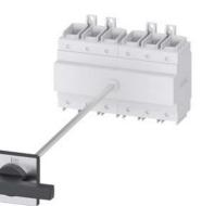
SENTRON, Switch disconnector 3LD, main switch, 6-pole, lu: 160 A, Operating power / at AC-23 A at 400 V: 75 kW, floor mounting with door coupling, knob-operated mechanism, black, 4-hole mounting of the handle
