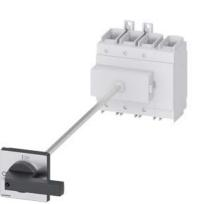
SENTRON, Switch disconnector 3LD, main switch, 4-pole, lu: 160 A, Operating power / at AC-23 A at 400 V: 75 kW, floor mounting with door coupling, knob-operated mechanism, black, 4-hole mounting of the handle
