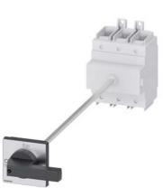
SENTRON, switch disconnector 3LD, main switch, 3-pole, lu: 160 A, operating performance / at AC-23 A at 400 V: 75 kW, floor mounting with door coupling, knob-operated mechanism, black, 4-hole mounting of the handle,
