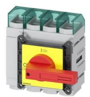
SENTRON, Switch disconnector 3LD, emergency switching-off switch, 4- pole, lu: 160 A, operating power / at AC-23 A 400 V: 75 kW, front-mounted, knob-operated mechanism, red/yellow, 4-hole mounting of the handle
