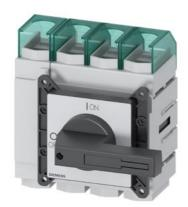
SENTRON, Switch disconnector 3LD, main switch, 4-pole, lu: 160 A, Operating power / at AC-23 A at 400 V: 75 kW, front-mounted, knob-operated mechanism, black, 4-hole mounting of the handle
