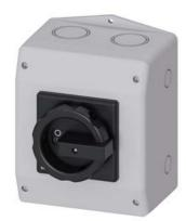
SENTRON, Switch disconnector 3LD, main switch, 6-pole, Iu: 32 A, Operating power / at AC-23 A at 400 V: 11.5 kW, molded-plastic encapsulation for metric screw connection, 1 NC, 1 NO, rotary operating mechanism, black
