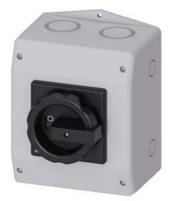
SENTRON, Switch disconnector 3LD, main switch, 6-pole, lu: 32 A, Operating power / at AC-23 A at 400 V: 11.5 kW, molded-plastic encapsulation for metric cable gland, rotary operating mechanism, black
