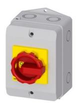
SENTRON, Switch disconnector 3LD, emergency switching-off switch, 3- pole, lu: 32 A, operating power / at AC-23 A 400 V: 11.5 kW, molded-plastic encapsulation for inch screw connection 4 NO, rotary operating mechanism, red/yellow
