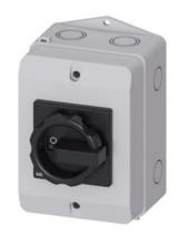
SENTRON, Switch disconnector 3LD, main switch, 3-pole, lu: 32 A, Operating power / at AC-23 A at 400 V: 11.5 kW, molded-plastic encapsulation for inch screw connection 4 NO, rotary operating mechanism, black
