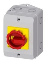
SENTRON, Switch disconnector 3LD, emergency switching-off switch, 3- pole, lu: 32 A, operating power / at AC-23 A 400 V: 11.5 kW, molded-plastic encapsulation for inch cable gland, 1 NC, 1 NO, rotary operating mechanism, red/yellow
