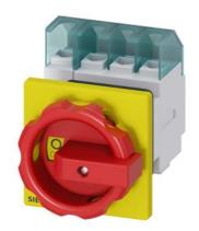
SENTRON, Switch disconnector 3LD, emergency switching-off switch, 4- pole, lu: 32 A, operating power / at AC-23 A 400 V: 11.5 kW, front-mounted, rotary operating mechanism, Red / yellow, central mounting 22.5 mm of the handle
