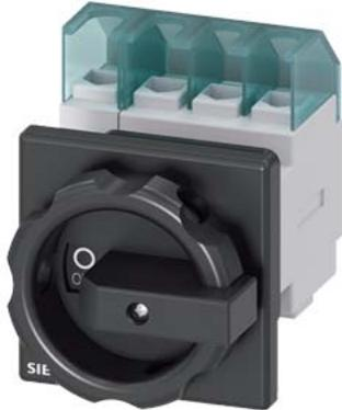
SENTRON, Switch disconnecter 3LD, main switch, 4-pole, Iu: 32 A, Operating power / at AC-23 A at 400 V: 11.5 kW, front-mounted, rotary operating mechanism, black, central mounting 22.5 mm of the handle
