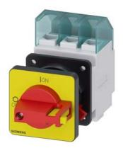
SENTRON, Switch disconnector 3LD, emergency switching-off switch, 3- pole, lu: 32 A, operating power / at AC-23 A 400 V: 11.5 kW, front-mounted, knob-operated mechanism, Red / yellow, central mounting 22.5 mm of the handle
