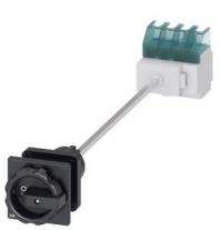
SENTRON, Switch disconnector 3LD, main switch, 4-pole, lu: 32 A, Operating power / at AC-23 A at 400 V: 11.5 kW, floor mounting with door coupling, rotary operating mechanism, black, central mounting 22.5 mm of the handle
