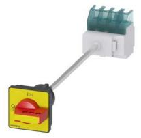
SENTRON, switch disconnector 3LD, EMERGENCY OFF switch, 4-pole, lu: 32 A, Operating power / at AC-23 A at 400 V: 11.5 kW, floor mounting with door coupling, defeatable knob-operated mechanism, red/yellow, 4-hole mounting of the handle
