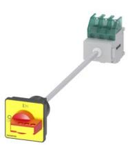
SENTRON, switch disconnector 3LD, EMERGENCY OFF switch, 3-pole, Iu: 32 A, Operating power / at AC-23 A at 400 V: 11.5 kW, floor mounting with door coupling, defeatable knob-operated mechanism, red/yellow, 4-hole mounting of the handle
