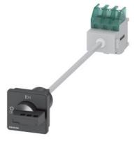
SENTRON, switch disconnector 3LD, main switch, 3-pole, lu: 32 A, operating power / at AC-23 A at 400 V: 11.5 kW, floor mounting with door coupling, defeatable knob-operated mechanism, black, 4-hole mounting of the handle
