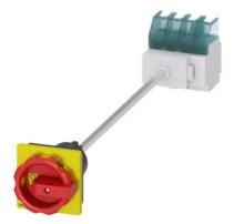
SENTRON, Switch disconnector 3LD, emergency switching-off switch, 4- pole, lu: 32 A, operating power / at AC-23 A 400 V: 11.5 kW, floor mounting with door coupling, rotary operating mechanism, Red / yellow, 4-hole mounting of the handle
