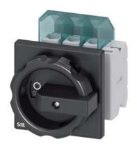
SENTRON, Switch disconnector 3LD, main switch, 3-pole, lu: 32 A, Operating power / at AC-23 A at 400 V: 11.5 kW, front-mounted, 1 NC, 1 NO, rotary operating mechanism, black, 4-hole mounting of the handle
