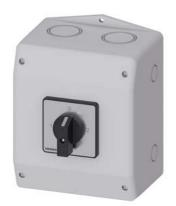
SENTRON, Switch disconnector 3LD, change-over switch, 3-pole, lu: 25 A, Operating power / at AC-23 A at 400 V: 9.5 kW, molded-plastic encapsulation for metric cable screw connection, knob-operated mechanism, black
