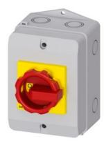
SENTRON, Switch disconnector 3LD, emergency switching-off switch, 3- pole, lu: 25 A, operating power / at AC-23 A 400 V: 9.5 kW, Molded plastic encapsulation for inch cable gland, 1 NC, 1 NO, rotary operating mechanism, red/yellow
