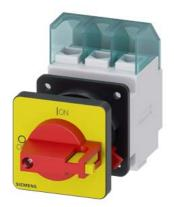
SENTRON, Switch disconnector 3LD, emergency switching-off switch, 3- pole, lu: 25 A, operating power / at AC-23 A 400 V: 9.5 kW, front-mounted, knob-operated mechanism, Red / yellow, central mounting 22.5 mm of the handle
