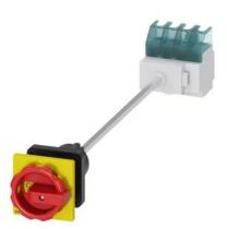
SENTRON, Switch disconnector 3LD, emergency switching-off switch, 4- pole, lu: 25 A, operating power / at AC-23 A 400 V: 9.5 kW, floor mounting with door coupling, rotary operating mechanism, Red / yellow, central mounting 22.5 mm of the handle
