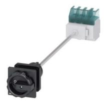
SENTRON, Switch disconnector 3LD, main switch, 4-pole, lu: 25 A, Operating power / at AC-23 A at 400 V: 9.5 kW, floor mounting with door coupling, rotary operating mechanism, black, central mounting 22.5 mm of the handle
