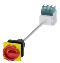
SENTRON, Switch disconnector 3LD, emergency switching-off switch, 3- pole, lu: 25 A, operating power / at AC-23 A 400 V: 9.5 kW, floor mounting with door coupling, rotary operating mechanism, Red / yellow, central mounting 22.5 mm of the handle
