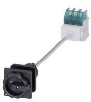
SENTRON, Switch disconnector 3LD, main switch, 3-pole, lu: 25 A, Operating power / at AC-23 A at 400 V: 9.5 kW, floor mounting with door coupling, rotary operating mechanism, black, central mounting 22.5 mm of the handle
