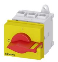
SENTRON, Switch disconnector 3LD, emergency switching-off switch, 3- pole, lu: 25 A, operating power / at AC-23 A 400 V: 9.5 kW, installation in distribution boards, knob-operated mechanism, Red / yellow, handle direct at the switch
