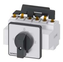
SENTRON, Switch disconnector 3LD, change-over switch, 3-pole, lu: 25 A, Operating power / at AC-23 A at 400 V: 9.5 kW, Front mounting, knob-operated mechanism, black, 4-hole mounting of the handle
