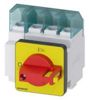
SENTRON, Switch disconnector 3LD, emergency switching-off switch, 4- pole, lu: 25 A, operating power / at AC-23 A 400 V: 9.5 kW, floor mounting with door coupling, knob-operated mechanism, red/yellow, 4-hole mounting of the handle
