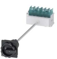
SENTRON, Switch disconnector 3LD, main switch, 6-pole, Iu: 25 A, Operating power / at AC-23 A at 400 V: 9.5 kW, floor mounting with door coupling, 1 NC, 1 NO, rotary operating mechanism, black, 4-hole mounting of the handle
