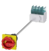
SENTRON, Switch disconnector 3LD, emergency switching-off switch, 4- pole, lu: 25 A, operating power / at AC-23 A 400 V: 9.5 kW, floor mounting with door coupling, rotary operating mechanism, Red / yellow, 4-hole mounting of the handle
