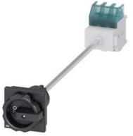
SENTRON, Switch disconnector 3LD, main switch, 3-pole, lu: 25 A, Operating power / at AC-23 A at 400 V: 9.5 kW, floor mounting with door coupling, rotary operating mechanism, black, 4-hole mounting of the handle
