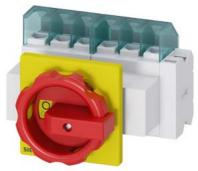
SENTRON, Switch disconnector 3LD, emergency switching-off switch, 6- pole, lu: 25 A, operating power / at AC-23 A 400 V: 9.5 kW, front-mounted, 1 NC, 1 NO, rotary operating mechanism, Red / yellow, 4-hole mounting of the handle
