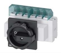
SENTRON, Switch disconnector 3LD, main switch, 6-pole, lu: 25 A, Operating power / at AC-23 A at 400 V: 9.5 kW, front-mounted, 1 NC, 1 NO, rotary operating mechanism, black, 4-hole mounting of the handle
