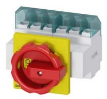
SENTRON, Switch disconnector 3LD, emergency switching-off switch, 6- pole, lu: 25 A, operating power / at AC-23 A 400 V: 9.5 kW, front-mounted, rotary operating mechanism, Red / yellow, 4-hole mounting of the handle
