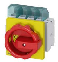
SENTRON, Switch disconnector 3LD, emergency switching-off switch, 4- pole, lu: 25 A, operating power / at AC-23 A 400 V: 9.5 kW, front-mounted, 1 NC, 1 NO, rotary operating mechanism, Red / yellow, 4-hole mounting of the handle
